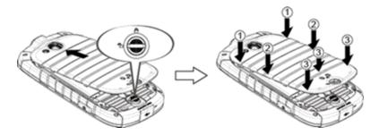
• Turn the battery cover lock clockwise to the locked position.
