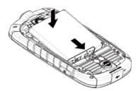
Replace the battery cover, making sure all the tabs are secure and there are no gaps around the cover.
