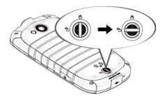
• Insert your thumb or fingernail into the slot and lift the battery cover gently.
