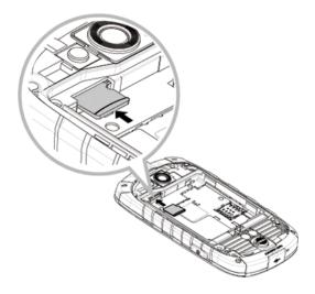
4. Replace the battery and the battery cover. See Insert and Charge the Battery.
