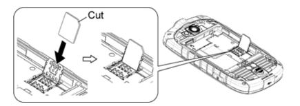
5. Replace the flap of the SIM card holder and slide the flap in the direction of the arrow to lock it.
